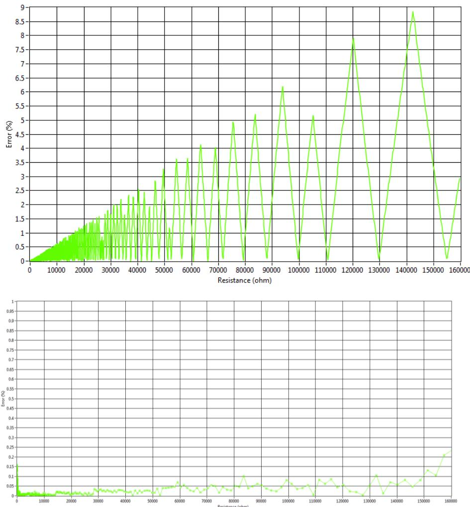
Users can estimate the accuracy for a given setpoint by reading out the actual resistance set by the device via USB (see *ReadResistanceOutput* in the software chapter). This value is the best permutation of the resistors that the device could find.
